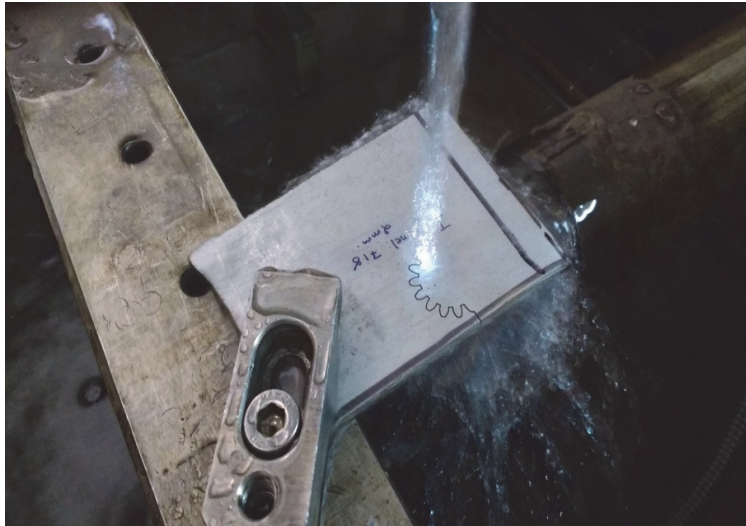
Fig. 1. Machining of the work-piece material by Wire EDM
