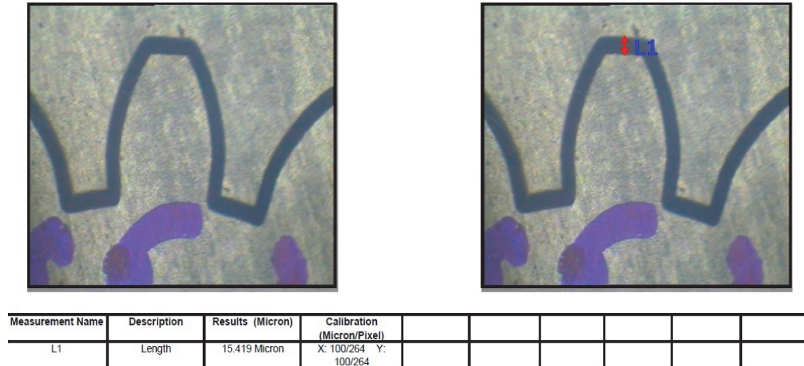
Fig. 2. Work-piece observed under optical microscope at 20X zoom
