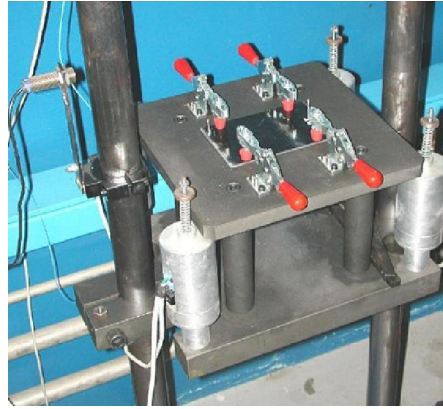
Fig. 3. Drop weight machine
