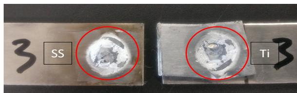
**Fig. 3.** Faying surface appearance of the welded joint.
