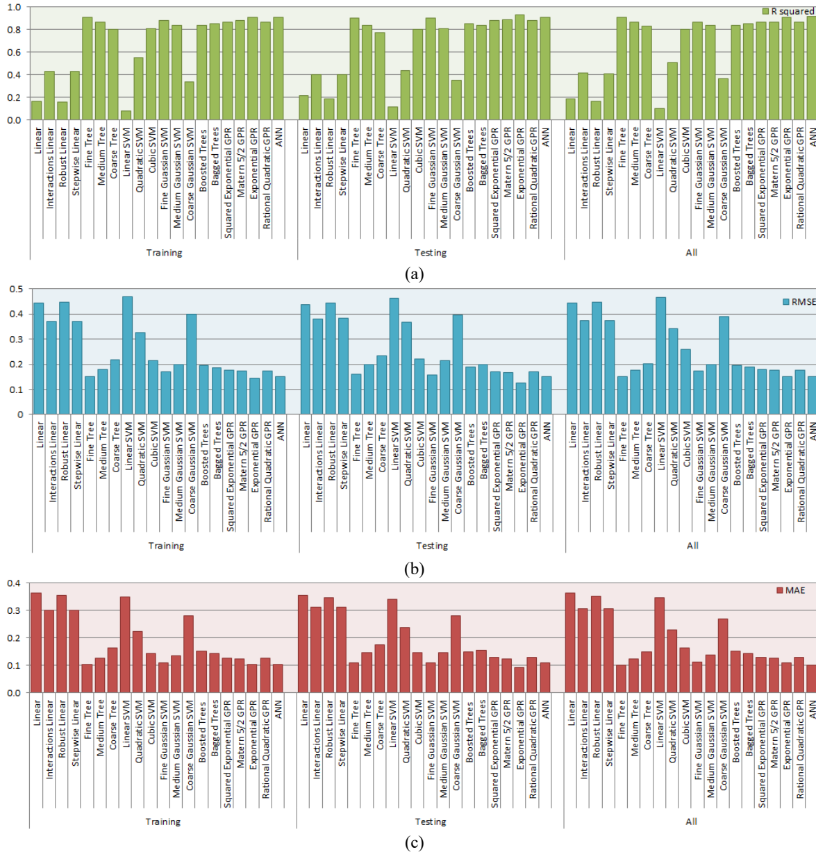
Fig. 3 Performance indices of the bead depth prediction for each model in terms of (a) R^2 , (b) RMSE, and (c) MAE
