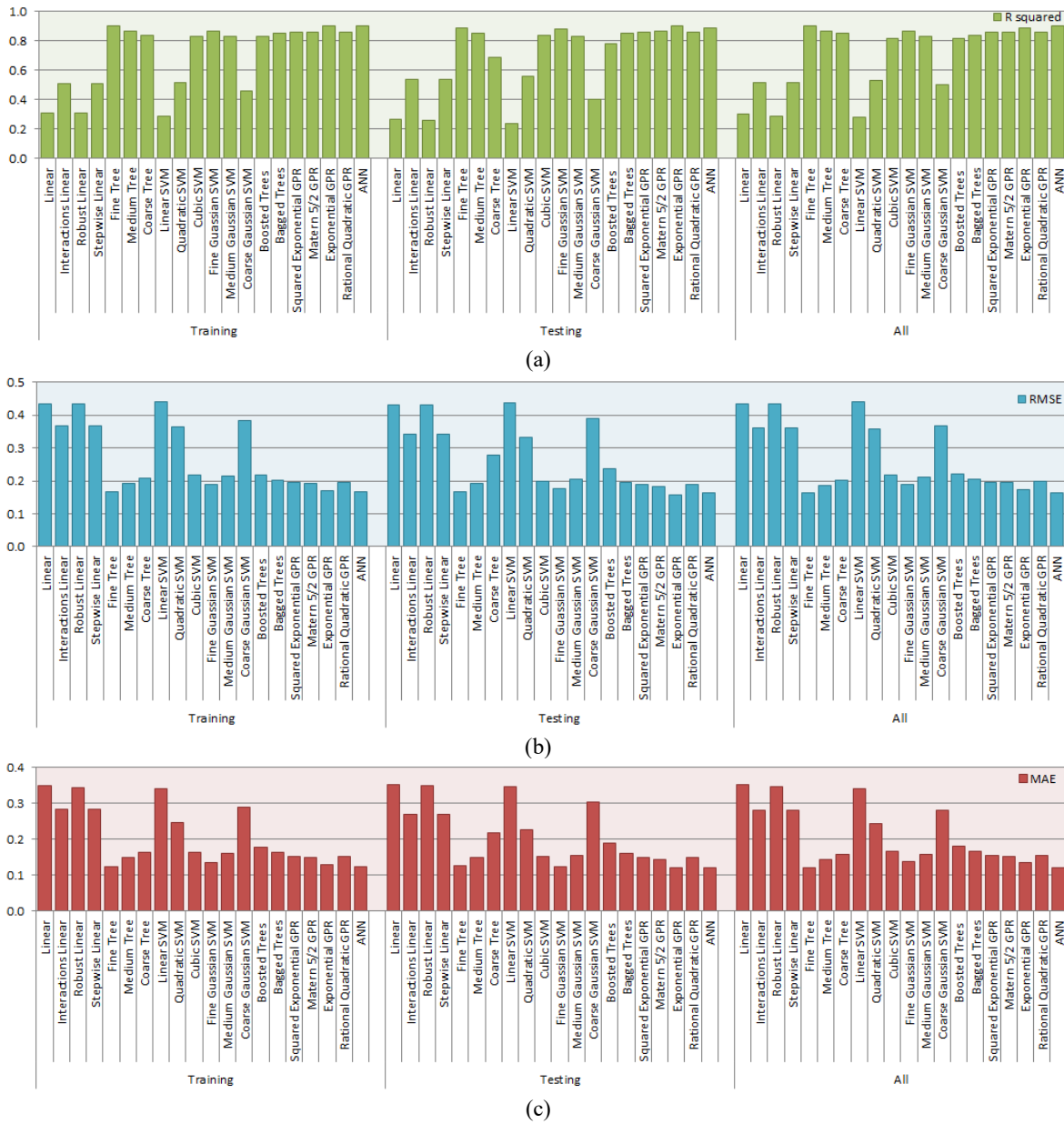
Fig. 4 Performance indices of the bead height prediction for each model in terms of (a) R^2 , (b) RMSE, and (c) MAE
