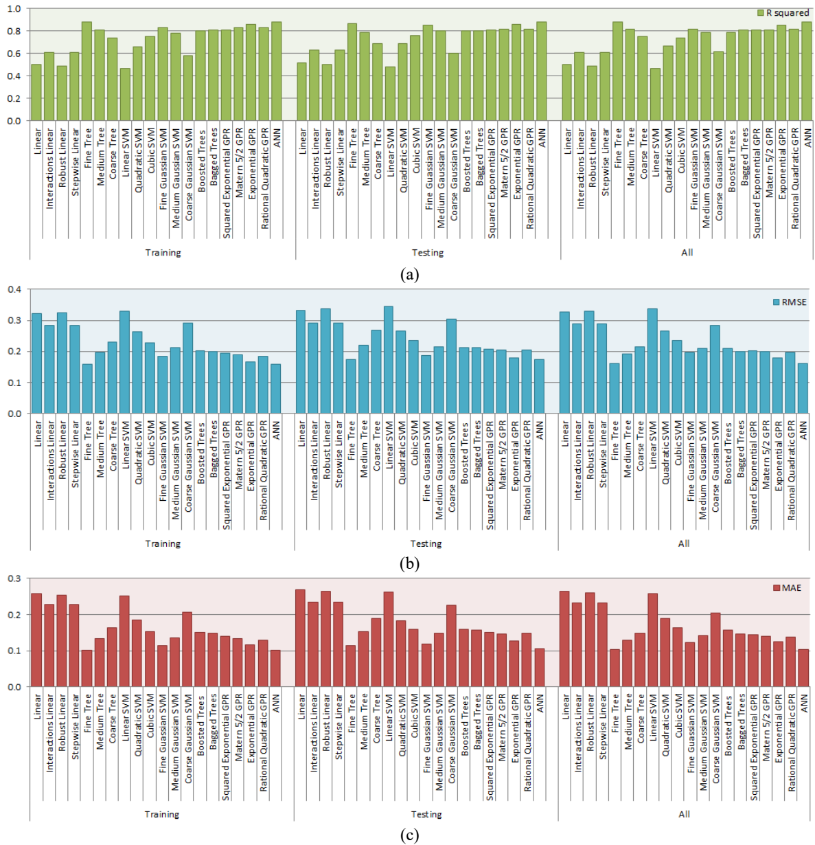
Fig. 5 Performance indices of the bead width prediction for each model in terms of (a) R^2 , (b) RMSE, and (c) MAE
