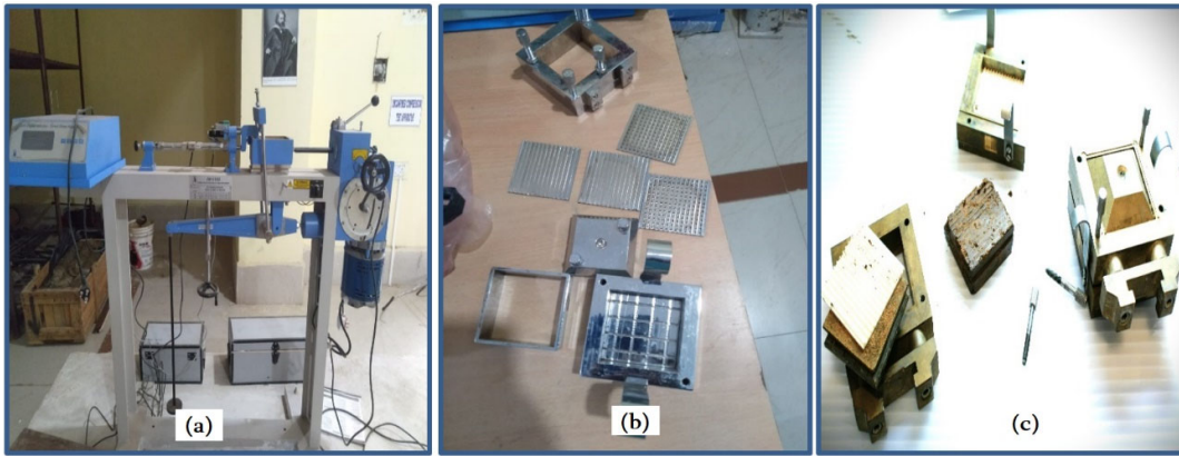
Fig. 2. (a) Direct Shear Testing Machine, (b) Shear box, and (c) Sample after testing
