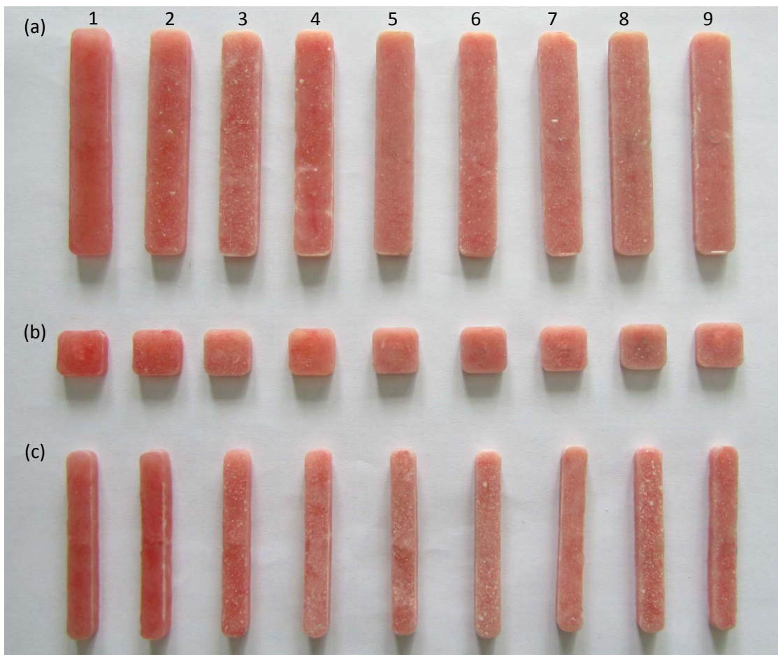
Fig. 2. Standard test samples a) flexural test, b) hardness and c) impact test
