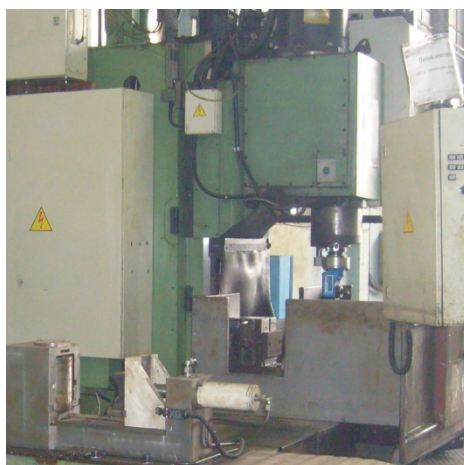
Fig. 3. Processing of rail-end-bolt holes on machine tool in FAE Sofia
