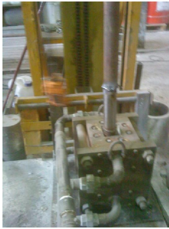
Fig. 1. ESR device used for specimens manufacturing
