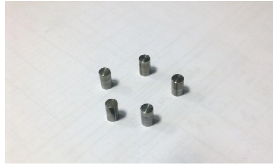
Fig. 2. Hot compression test specimens before testing
