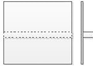
Fig. 2. Geometry of eccentrically stiffened isotropic plate
