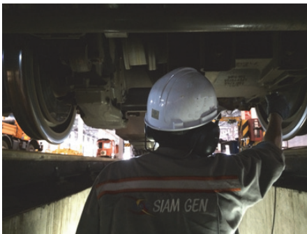
Fig. 3. Experimental set up for TBU bearing fault detection using AE
