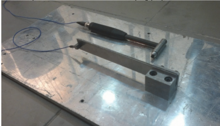
Fig. 3. A setup assembly to examine vibration-damping properties of the viscoelastic material
