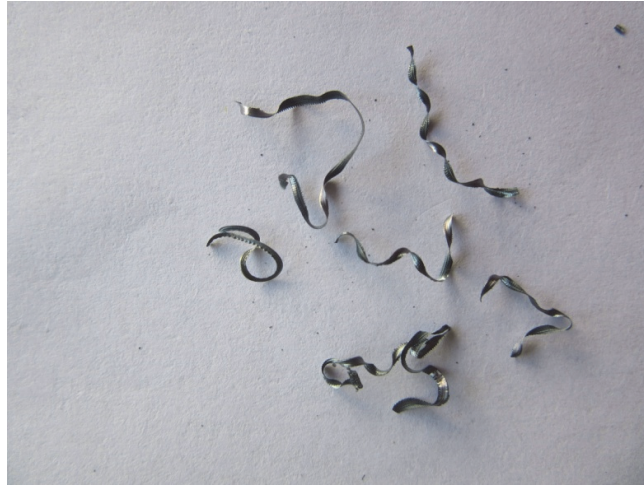
Fig. 3. Image of chips at Run 7 ( v = 190 m/min, f = 0.12 mm/rev and d = 0.2 mm)
