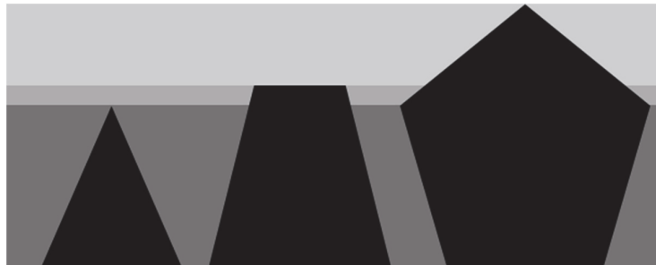
Fig. 5. Simultaneous build-up of multiple parts with different heights
